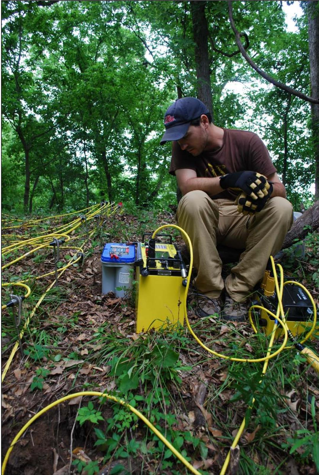
Figure 5. ERT data collection with AGI 56 probe SuperSting R8 IP eight-channel memory earthen resistivity meter in process. Photograph by Megan Kassabaum.
